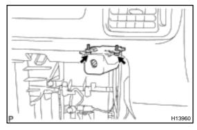
(d) Install the passenger airbag manual on–off switch with the 2 bolts.
