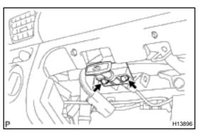
(e) Install the hood release lever with the 2 bolts.
